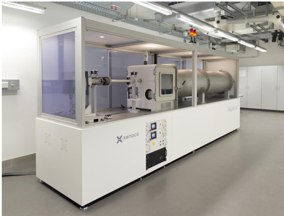
Data collection with the MAUS SAXS/WAXS instrument
